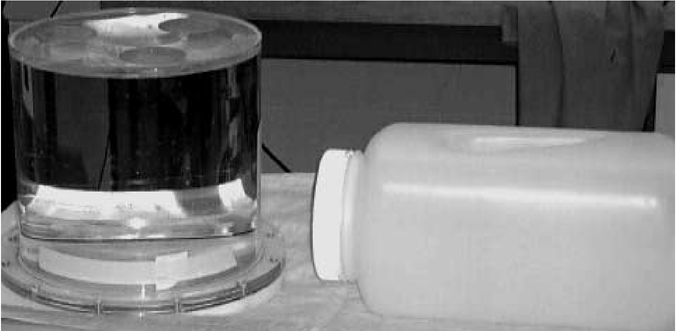
Illustration 2-4 FLOOD AND BOTTLE PHANTOM SIMULATING A WHOLE BODY STUDY
